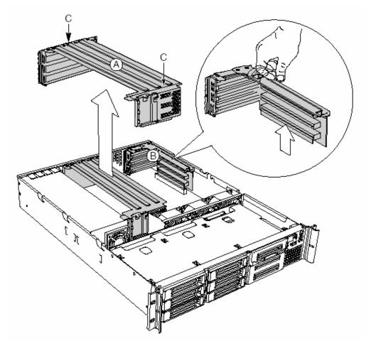
Figure 9: Removing the Riser Cards
